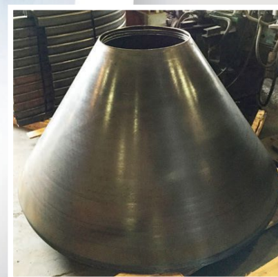
5/16" plate cone with a 16" minor diameter and a 48" major diameter with an overall height of 42"
