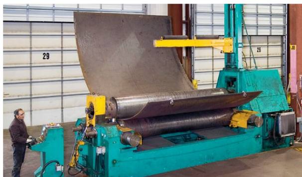
2" x 12' plate roll can roll 40' lengths
