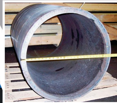
1 1/2" plate 45" long rolled to a 25" inside diameter
