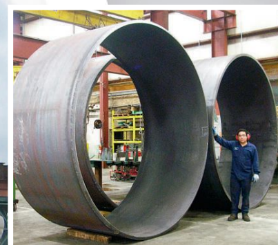
2" x 58 1/2" beveled plate rolled to a 128" outside diameter
